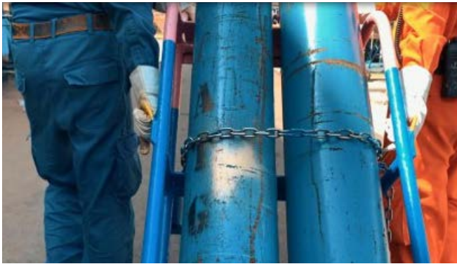
Handles to manoeuvre the gas cylinder trolley
