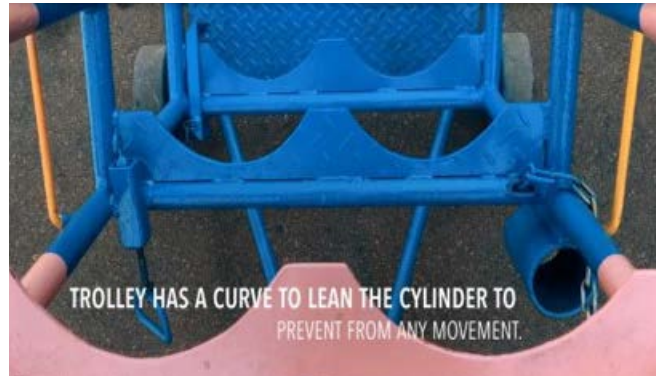
Cylinder placeholder to prevent movement
